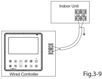
The main/secondary wired controller can be used to enable two wired controllers to control one unit, and the wired controllers connect to the unit HA and HB ports through the HA and HB port on the controller. There is no polarity
