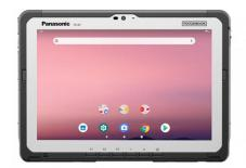
**TOUGHBOOK A3.** This rugged Android 10.1" has all the features of the 7" S1 tablet, plus insertable stylus and optional barcode reader and insertable smart card reader, making it ideal for FSOs. Its outdoor-viewable display, featuring a 5' foot drop rating and IP65 certification for dust and water resistance make the TOUGHBOOK A3 the right rugged device to get more out of every FSO technician's day.
