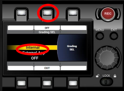
2. Press Grading SEL Use dial and select Internal, Press Dial to confirm
