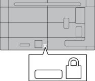
The display has holes for attaching eyebolts (M10). When installing, use them to suspend the display.
