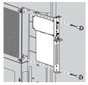
Tightening torque guideline: 0.5 N·m or less
