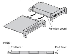
3 Using the screw removed in step 1, fix the function board to the SLOT adaptor.
