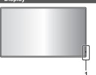
1 Power Indicator / Remote control sensor The Power Indicator will light.
