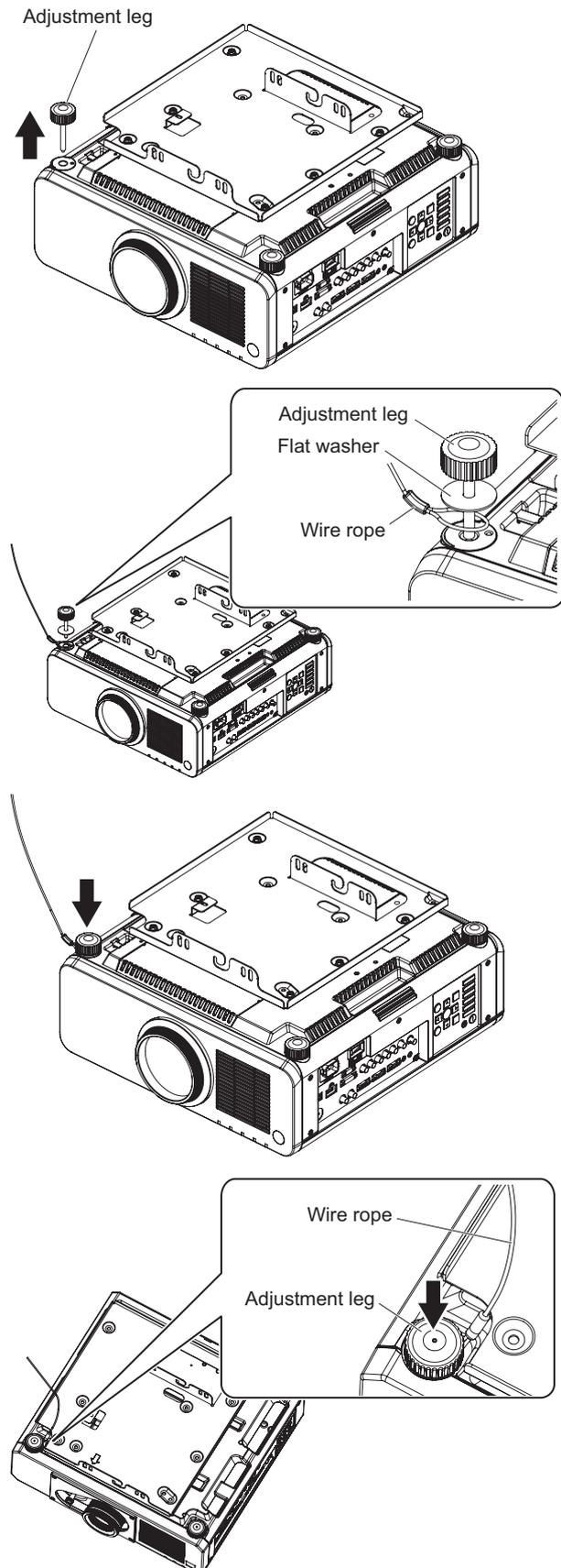
1) Turn the adjustment leg (one) counterclockwise to remove it from the projector.
