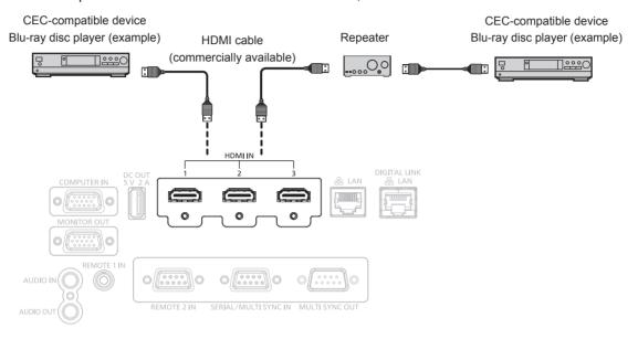
Connection example with CEC-compatible device
