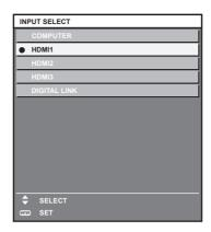
2) Press ▲▼ to select the input for projection, and press the <ENTER> button.
