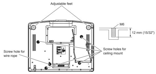
Positions of screw holes for ceiling mount and adjustable feet
