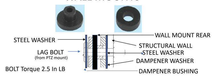
THE **FEC-VIBDAM1** VIBRATION DAMPENER KIT ASSISTS IN REDUCING YOUR PTZ CAMERA FROM UNWANTED VIBRATION WHEN INSTALLED ON ANY CURRENT **FEC** PTZ WALL MOUNT.
