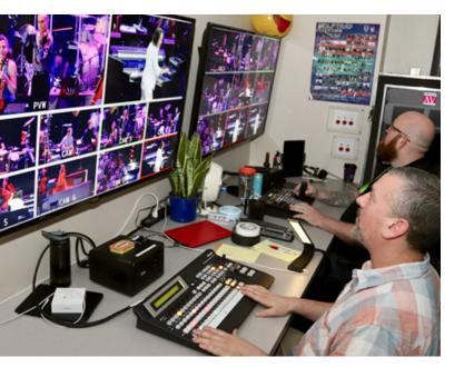
The AV-HS450 switcher is located in a new camera control center under the stage.
