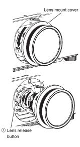
Turn the lens mount cover counterclockwise to detach it from the lens and slide it towards the front end of the lens.
