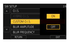
First, there's an overall on/off setting for the Custom O.I.S. system. If you set "CUSTOM O.I.S." to OFF, then the default optical image stabilization parameters will be used. If you want to take advantage of your customized settings, you need to set this to ON.
