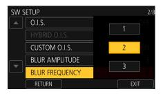
The second major parameter you can adjust in the O.I.S. system is the BLUR FREQUENCY. The frequency refers to how frequently the camera can expect to encounter unwanted motions that it should attempt to stabilize. Unlike BLUR AMPLITUDE, this setting isn't directly proportional to its effect; instead, there are three different "personalities" you can ask the camera to adopt.
