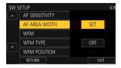
Finally, there is a fourth parameter you can control regarding the focus system, and that's the size of the area in the frame that the autofocus system will evaluate for focus purposes. You can use the AF AREA WIDTH menu item to set how wide, or how narrow, the area it will evaluate will be.
