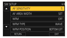
The second major parameter that you can customize is the AF SENSITIVITY. This parameter governs the autofocus system's responsiveness to initiating a refocus procedure (i.e., it controls how "sensitive" the autofocus system is towards thinking it needs to refocus the image). The range of settings are from 0 to 10, and the default setting is at 5.
