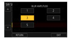
There are two major parameters you can set for the custom O.I.S. system, BLUR AMPLITUDE and BLUR FREQUENCY. Blur amplitude refers to how large the motion is that the O.I.S. system will be working with; the bigger the movement, the more "ample" it is. The blur amplitude has five options; the smaller the number you set it to, the smaller the movements that the O.I.S. system
