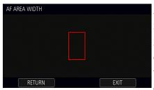
Alternatively, you can set the frame to be narrower, even to a very narrow degree. The image to the left shows the focus frame at its most narrow. In this setting, the camera will ignore everything outside the red frame, and will only determine focus on what is within that red frame; this small size might be useful to isolate one player out of the whole line of players, and keep that player in
