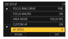
Once you've enabled the CUSTOM AF option, the first customizable parameter is AF SPEED. This governs how quickly (or slowly) the autofocus motor works. The range is from -5 to +5, with 0 as the default setting.
